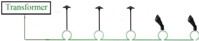
Cut and splice with wire connectors at each fixture
